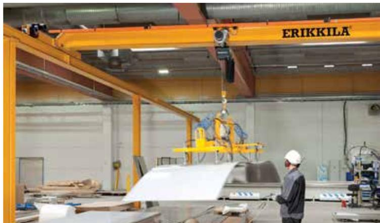
SPARTAN Bridge Crane is a complete "Tailored system" for the industry. With a span up to 18 meter. Capacity from 1,6 to 10 ton. SPARTAN can be offered with electrical chain hoist or wire rope hoist. Standard with pendant control. SPARTAN are easy to install.no welding movements. Minimized environment. SPARTAN is very competitive and price-wise.
