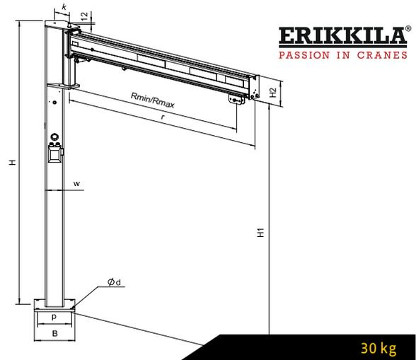
PELARSVÄNGKRAN / COLUMN MOUNTED JIB CRANE - LITTLE JOHN
